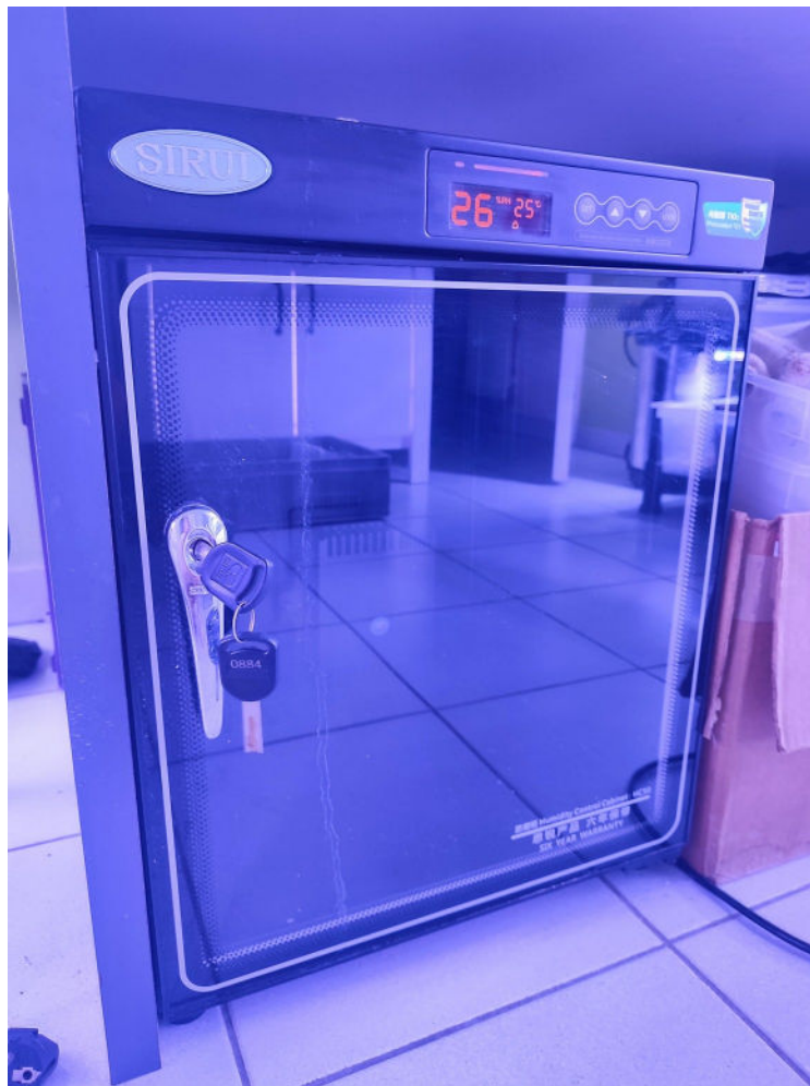
The SIRUI HC-40 I am using for drying pollen, the screen shows that RH is 26% and temperature 25°C
